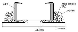
Attaching surface-mounted devices (SMDs) with electrically conductive adhesives is a commercially attractive method of component connection to supplement or even replace conventional soldering methods.
